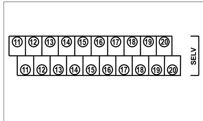
The connected devices or sensors must be suitable for SELV or marked with protection class III.
